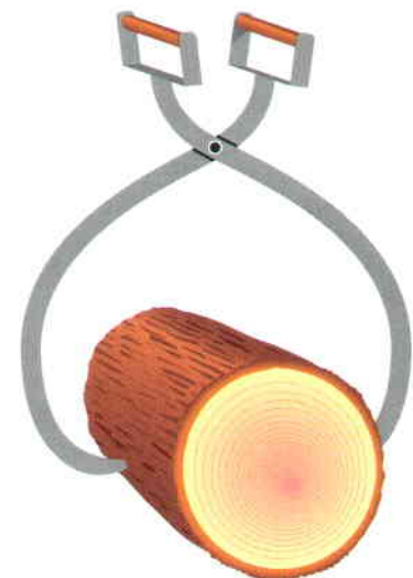
Figure 19-47 Timber tongs. Holding the handles together causes the claws to grip the log; and closing the claws on the log causes the handles to come together. Moreover, the greater the pull on the tongs, the tighter the grip at both ends. In an integrin molecule, the details of the linkage are different, but the mechanical principles are similar: conformational changes at opposite ends of the molecule are coupled, and pulling tightens the grip.
